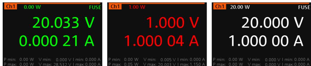
**Figure 5-3: Color coding of difference operating conditions**
