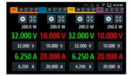
The Keysight E36200 power supplies have a 4.3" LCD color display.
